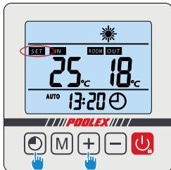
Press + simultaneously for 5s and the **SET** LED will flash quickly, indicating the control box is ready to be paired.
