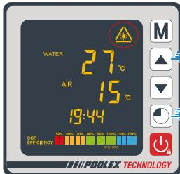
Press + simultaneously for 5s and the LED will flash quickly, indicating the control box is ready to be paired.
